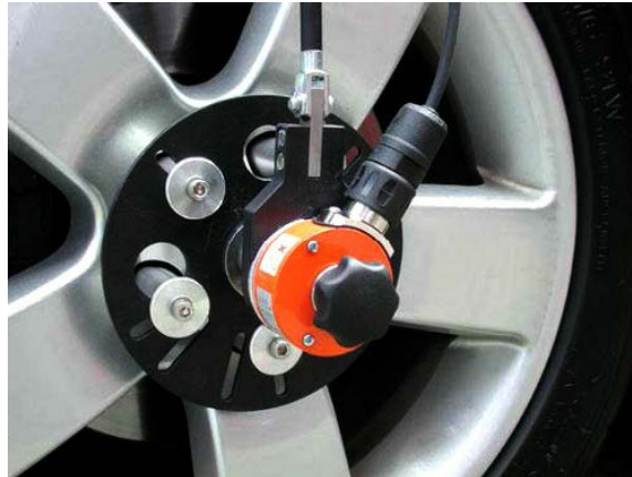
Image 93: Mounting preview of a wheel speed sensor
