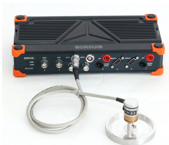
Image 4: Encoder connected to Dewesoft Sirius device
