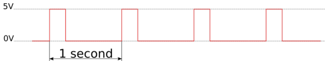
Image 22: Pulse per second signal (low and high voltages differ with implementation)
