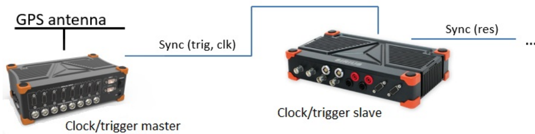
Image 37: GPS PPS connection example from Dewesoft device
