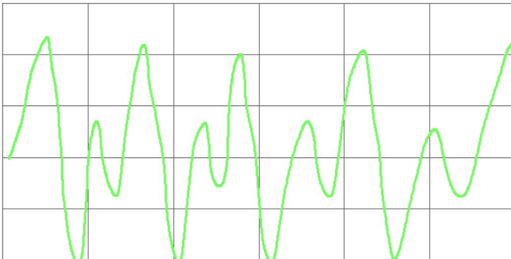
The time waveform plot will show both 1X vibration and a subsynchronous component near  $0.48X$  with an amplitude that varies over time
