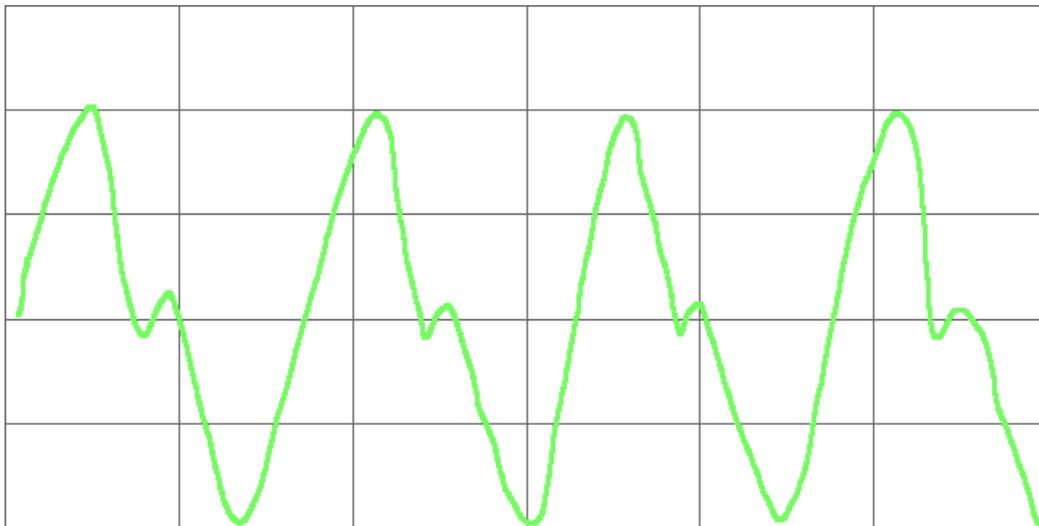
Misalignment will often result in a 2X response. This will be apparent in the direct waveform plot with an increase in peak-to-peak amplitude and 2X frequency component.
