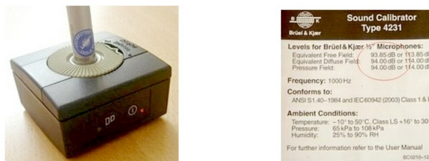
Image 25: Calibrating the microphone with the calibrator
