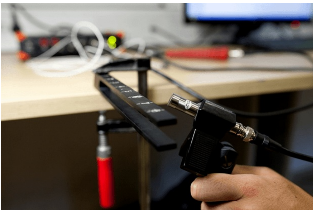
Image 33: Measurement of tuning fork vibrations with microphone
