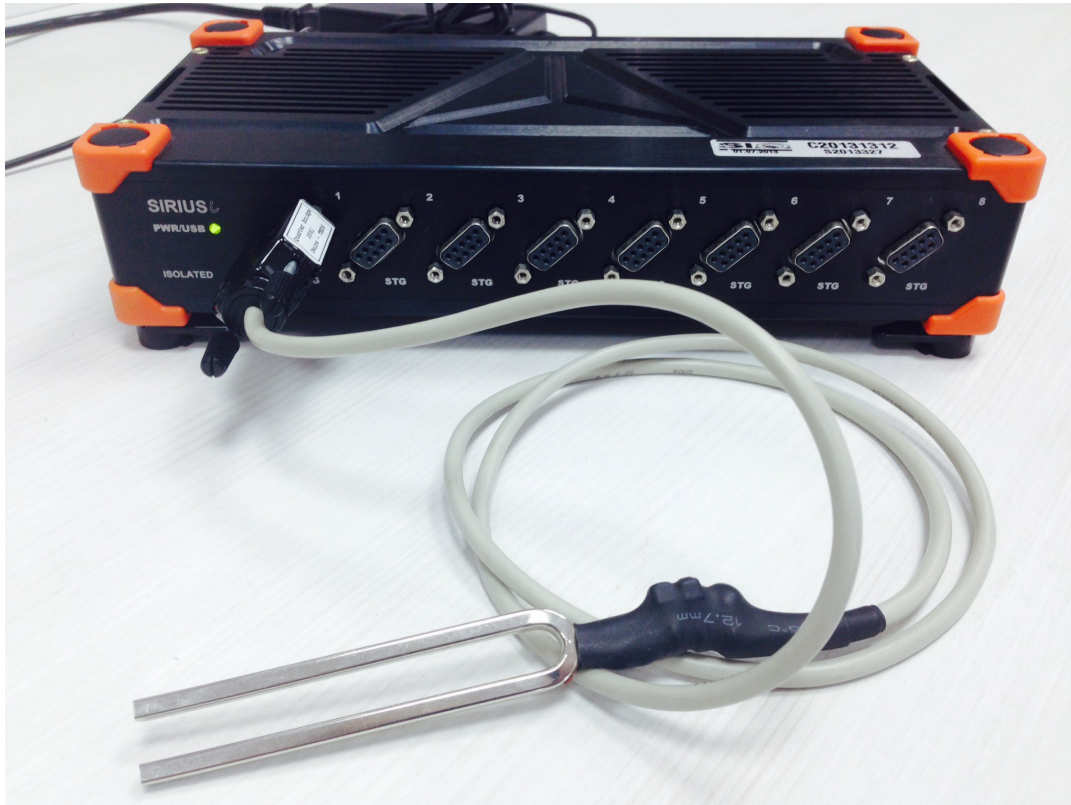
Image 25: Tuning fork connected to SIRIUS measurement system
