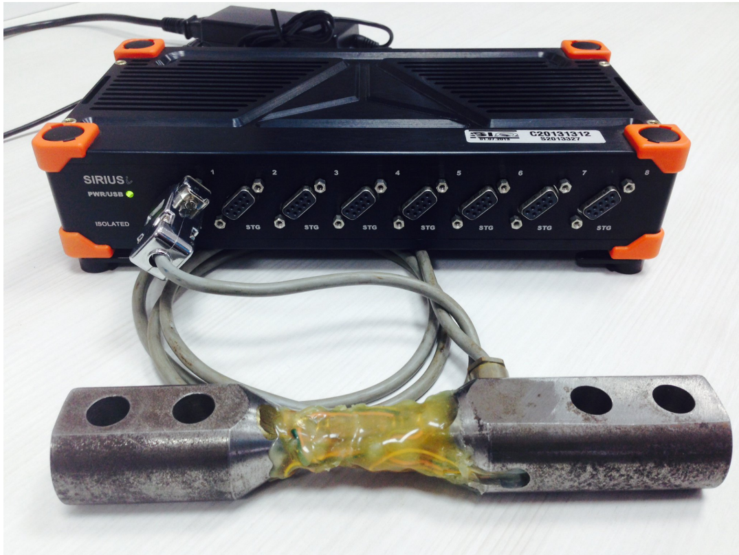
Image 41: Load cell connected to SIRIUS measurement system
