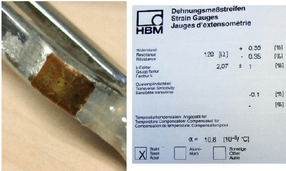
Image 26: Specifications of a strain gage
