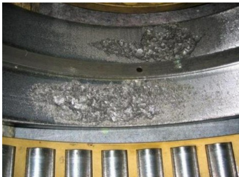
Image 52: Damaged outer ring of the large bearing
