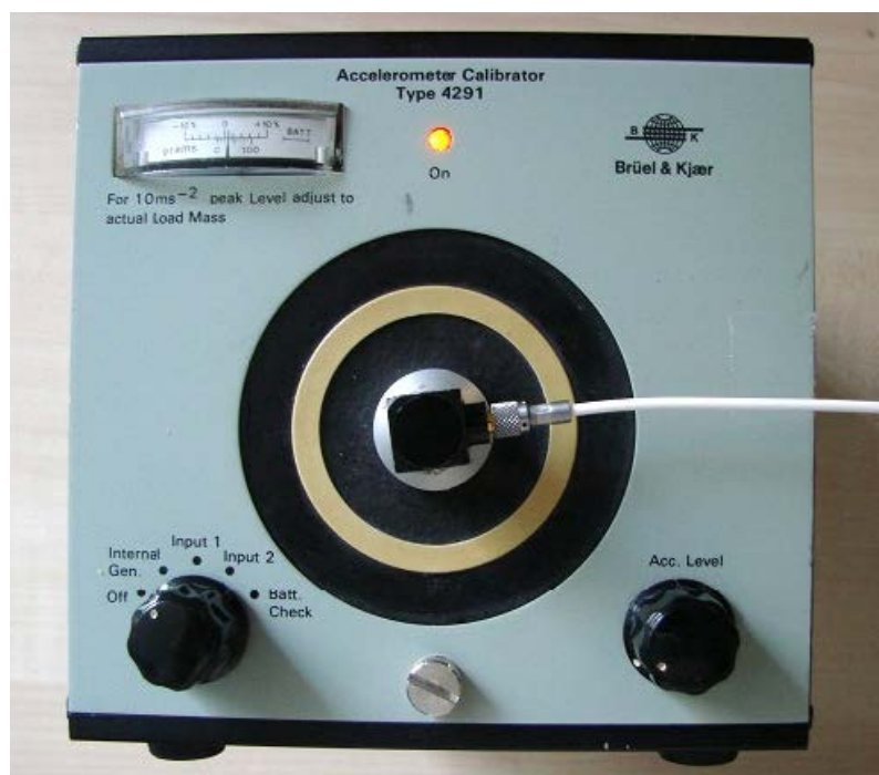
Image 29: Calibrator for accelerometers
