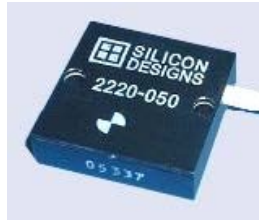
Image 21: An example of MEMS accelerometer
